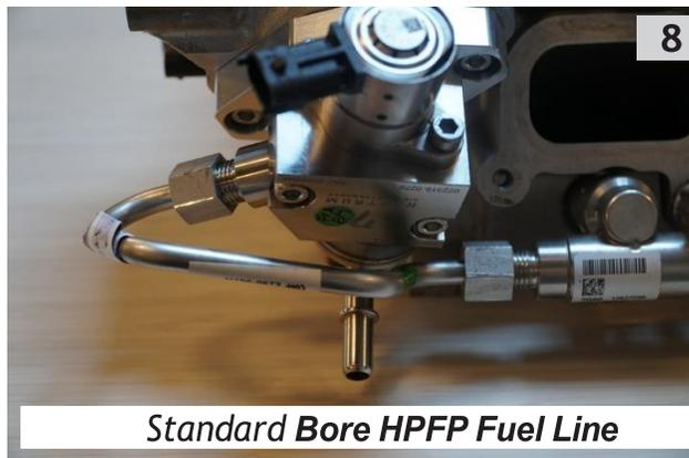
9. Attempt to move or shake the high-pressure hard line at both ends near the fittings. They should not move inside the compression nut. If they do move, remove the tube and go back to Step 7.
