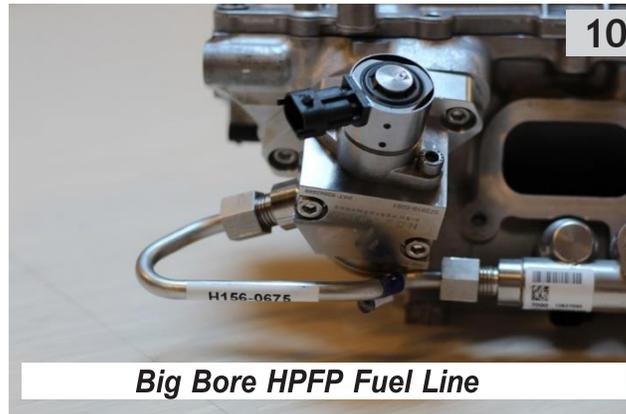
**NOTE: Standard bore kits and Big Bore Kits have different High Pressure tubes and Low Pressure adapters.**
