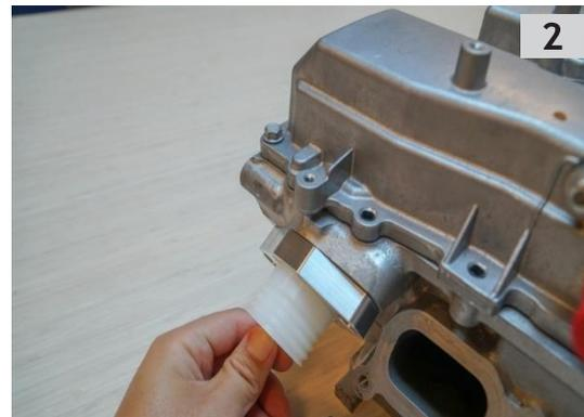
**TIP: Rotate the installation tool while seating the two fasteners. This will assist in preventing the installation tool from becoming trapped and difficult to remove.**
