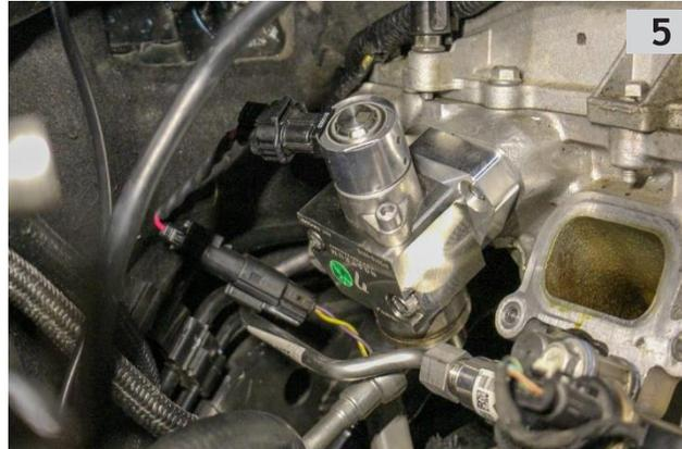
5. Obtain the electrical connector jumper from the kit. Plug the Molex male into the engine wire harness. Plug the Bosch Compact female to the male on the pump. Be sure, in both cases, that both connectors lock into the mating connector (you should hear a click). Check by pulling on the connectors. **Do not pull on the wires!!!**
