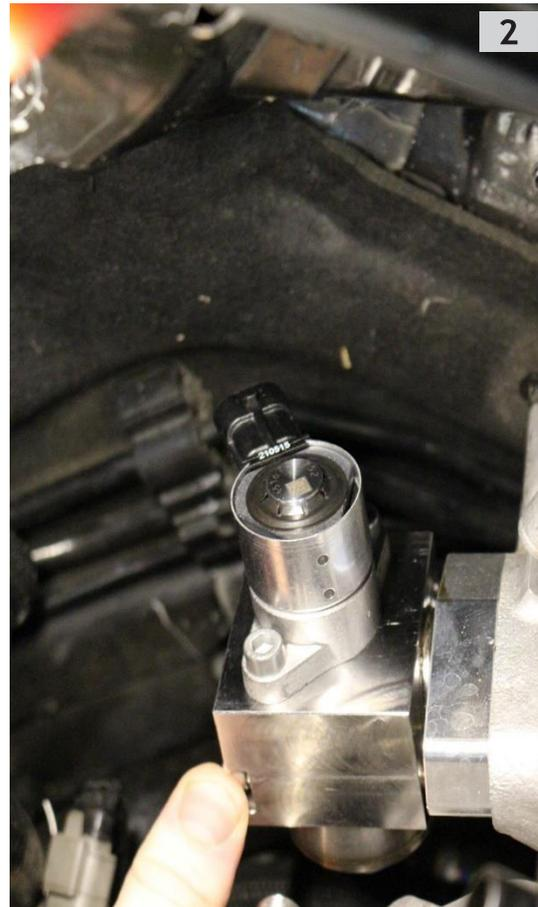
4. Push the pump deep into the flange until it seats against the flange face. Since your camshaft might not be at its base circle, you may need to gradually “walk” your pump in to load the return spring.
