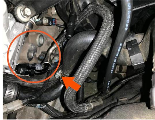
13. Reinstall your low-pressure fuel line to the **3/8"** quick connect male fitting. Make sure it is secure.
