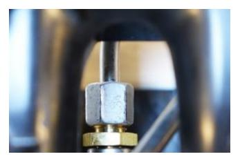
NOTE: You may need to remove the airbox and wiring harness clip to gain access to the fitting from underneath the intake manifold. This is the best way to get an open-end wrench to the fitting. See your OEM maintenance manual.
