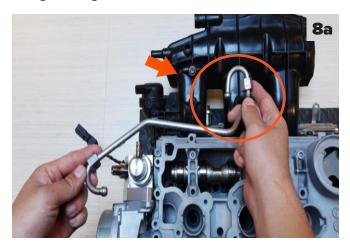
9. Next, ensure the spherical fitting is seated and aligned on the FUEL PUMP side. While holding the FUEL PUMP fitting in place, align the other end of the hard line spherical fitting to the FUEL RAIL female cone. IT IS IMPORTANT TO ENSURE THE FUEL PUMP FITTING IS SEATED FIRST, THEN SEAT THE FUEL RAIL SIDE.
