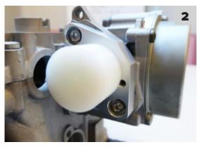
TIP: Rotate the installation tool while seating the two fasteners. This will assist in preventing the installation tool from becoming trapped and difficult to remove.
