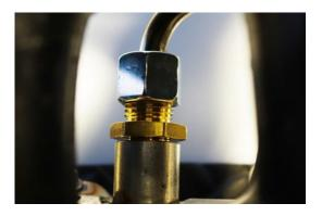
11. Attempt to move or shake the high-pressure hard line at both ends near the fittings. They should not move inside the compression nut. If they do move, remove the tube and go back to Step 8.
