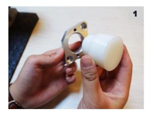
2. Insert the installation tool into the pump bore on the cylinder head (vacuum pump housing). Be sure to gently slide into the bore. The installation tool will align the flange and the O-ring into proper orientation and concentric alignment with the pump bore on the cylinder head. This prevents O-ring damage, pump damage, and pump installation problems. Push into the bore until the flange and O-ring are seated against the
