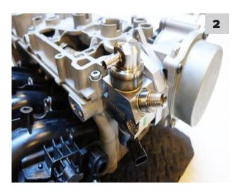
3. Obtain the two stainless steel M6  $\times$  45mm long Allen bolts from the kit and align the pump main body bolt holes to the threaded holes on the flange. Insert the bolts and hand start them.
