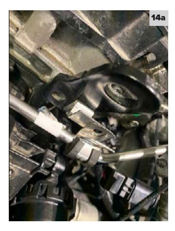
14. After tube is installed) Align the rubber-lined P-clamp with the "Z" bracket and fix them together with the provided M6 bolt & nut. Torque the bolt to 9 ft-lb. (See fig. 14a and 14b)
