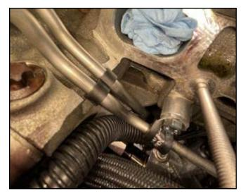
12. Install the feed line to vehicle fuel supply.
