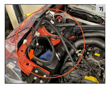
k. Remove the bolts for the intake manifold using a 11mm deep socket there will be some bolts and some nuts on the intake manifold.
