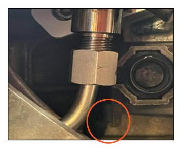
9. Install the high-pressure tube from pump two to the fuel rail. Place the bottom globe fitting in first. Make sure that the tube is tucked behind the wire harnesses. Once the globe fittings are both in place tighten the tubes finger tight then torque to 20 ft-lbs. using a 18mm crow foot on a torque wrench.
