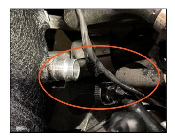
b. Remove the electrical connector from the evap. purge solenoid using a straight pick to pull up the metal clip and then pull on the connection.
