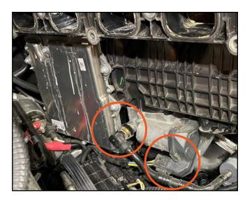
m. Fully remove the intake from the engine and place towels in the runners to prevent debris from getting in during install.
