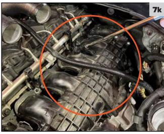
I. Start pulling the intake away from the engine straight out. Then once it clears the studs out towards the front of the car. Remove the throttle body connector while pulling and the evap. purge solenoid line. It helps to flip the manifold over to do this.
