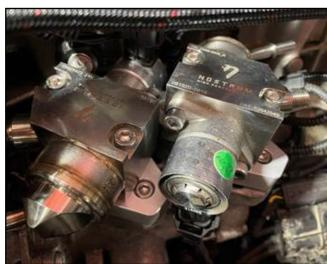
a. Place each pump into the engine. Begin with the front pump then install the rear pump. Using an extended 5mm Allen key, alternate between the two bolts fixing the flange to the engine to avoid damage. Once the bolts are seated down, torque the bolts that attach the flange to the engine to  $8.8~\mathrm{ft}$  – lbs.
