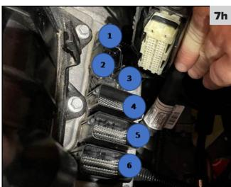
i. For the bulk connector numbered one above, reach around the intake to get access to the ECU and use a prying tool to pull out the U-clip. When the U-clip is fully pulled out to the position (shown below circled in blue), pull up on the connector to remove it from the ECU.
