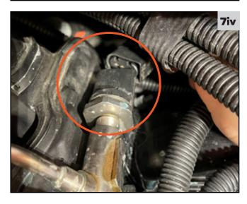
j. Remove the wiring harness out of the way of the intake manifold over towards the left of the car.
