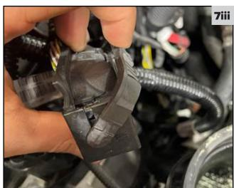
iv. Remove the electrical connector on the high-pressure fuel sensor located on the fuel rail towards the back of the engine. Squeeze on opposite sides of the connector on the wider portion to release it.
