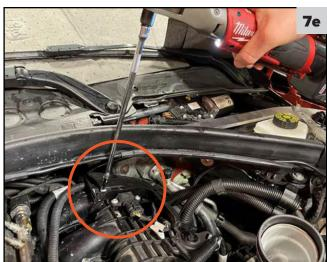
f. Remove the electrical harness routing connections from the bracket mentioned in the previous step
