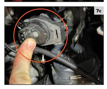
d. Remove the electrical connector from the cold air intake and the oil sensor using the straight pick.
