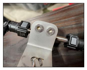
b. Attach two low pressure lines, the fuel feed tube and the tube that will connect to high-pressure fuel pump number two. Use the image below as reference.
