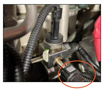
6. Install the high-pressure tube from pump one to the fuel rail. Place both globe fittings into the fuel rail then tighten each side finger tight. The globes should be seated but the tube should still be able to articulate.
