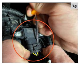
h. Remove the ECU bulk connectors. Follow the order numbered in the image below when disconnecting the connectors.
