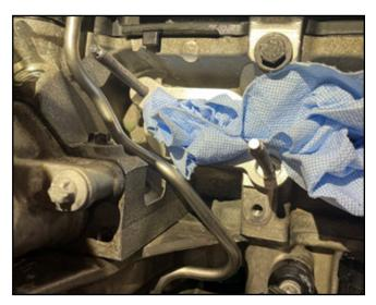
7. Once the tube is lightly in place, articulate the tube until there is no contact with the block or head of the engine. Once the tube is in place, tighten both lock nuts 20 ft-lbs using a 18mm crow's foot on a torque wrench.
