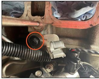
16. Remove the bolts that attach a mounting bracket to the back of the vacuum and pump housing using T30. You will need those bolts for installation of the upgraded high-pressure fuel pumps.
