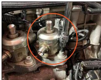
b. Remove both high-pressure pumps from the vehicle.
