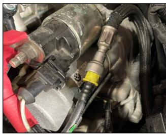
13. Install the low-pressure sensor connector to the new low-pressure sensor on the t-split.
