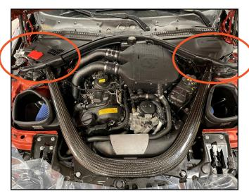
4. Remove the carbon sway bar using a T45 and 14mm Socket
