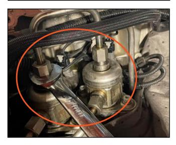
b. Remove the two bolts that are under the electrical housing that is right under the low-pressure sensor using a 14mm socket. Note: It will help if the socket is magnetic to avoid dropping the bolt into the undertray.
