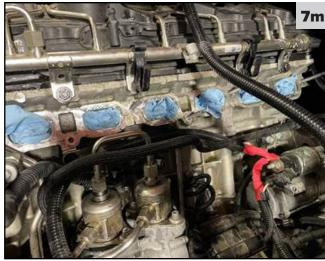
8. When the intake is out of the vehicle, check for dried coolant on the intake ports or intake manifold. This indicates a faulty charge air cooler. Make sure to replace it before proceeding with installation. BMW part number is 17517846235.
