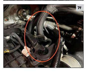
g. Remove the map sensor electrical plug from the intake manifold near the back of the motor.
