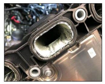
9. Check the valves for carbon build up. DI exclusive engines will leave carbon deposits on the back sides of the valves because no fuel is spraying on the back of the valves. Use CRC GDI Valve Cleaner. A tutorial on how to use the product can be found at the following link.
