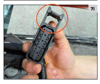
ii. Remove connector two and three by squeezing the sides of the connector then pulling up.
