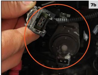
c. Pull the purge solenoid off the hanging bracket.
