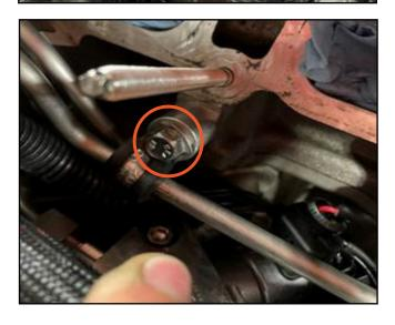
11. Install the W clip on the two tubes where they pass through the head to prevent the tubes from being able to contact the head during operation of the vehicle.
