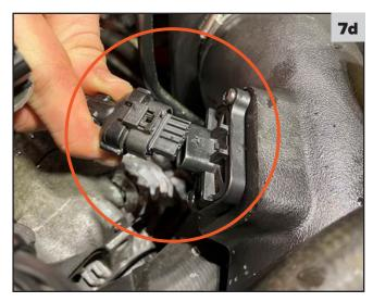
e. Remove the electrical connector bracket near the back of the engine on the intake manifold using the T25 bit with a 6-inch extension with swivel.
