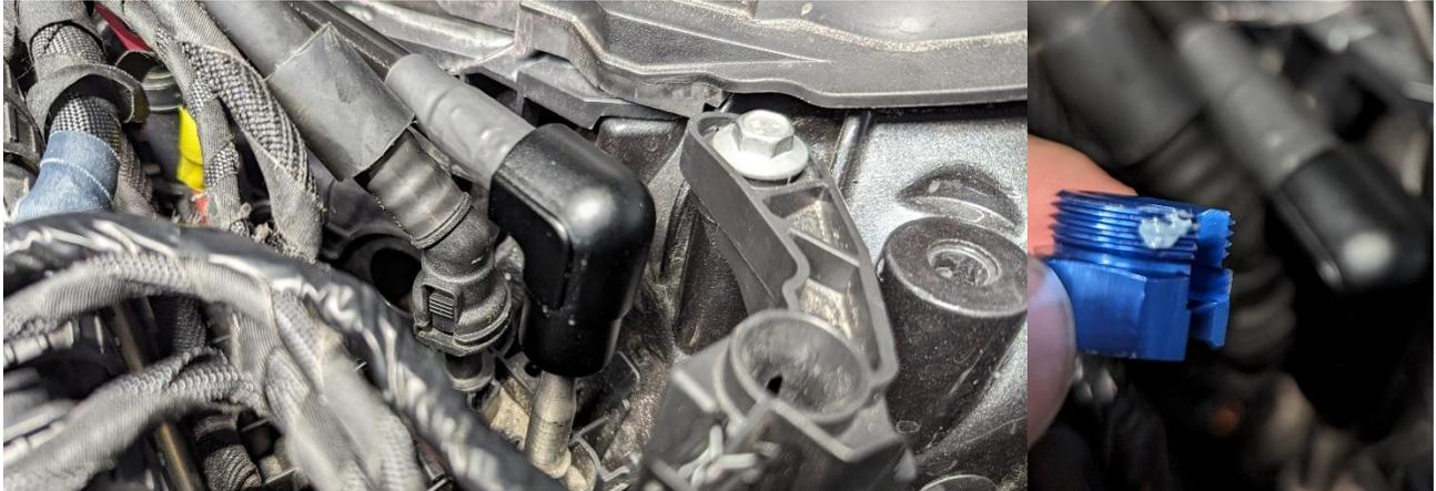
**CAUTION:** USE TWO HANDS WHEN THREADING THE BLUE COLLAR NUT. These can easily be dropped in the engine bay without using caution.
