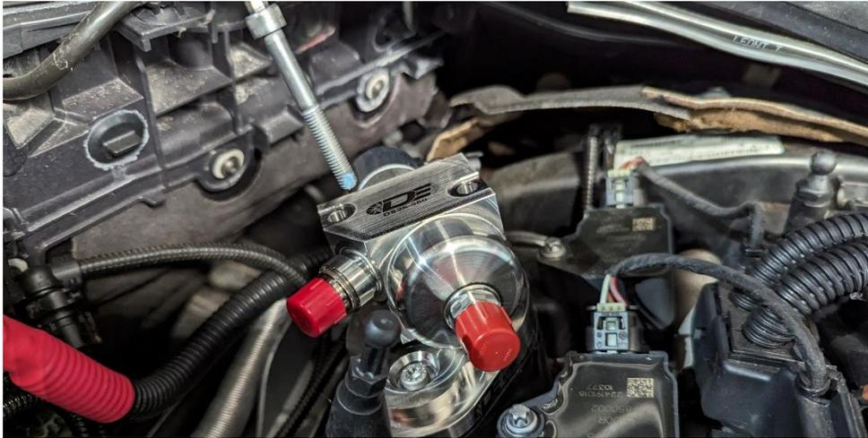
14. **READ THIS STEP THOROUGHLY.** Now install the supplied high pressure line. This line needs to be installed into the rear-most fuel rail port first, then rocked over into the fuel pump port, and lastly pulled down and back into the front-most fuel rail port. It will be a tight fit and the line **MUST BE AS STRAIGHT AS POSSIBLE**.
