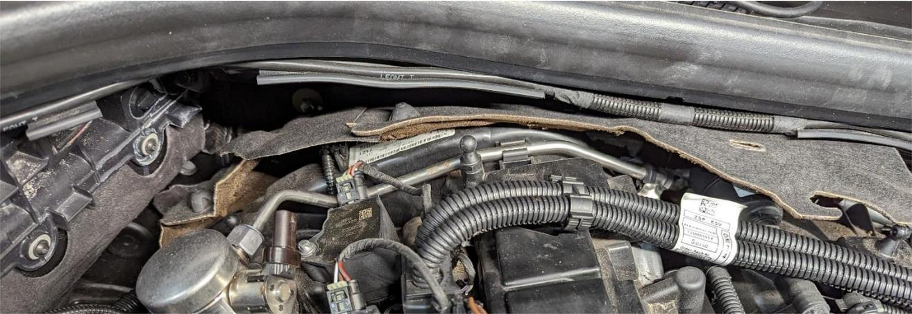
6. Next, using an E6 socket, remove the fastener which is securing the low pressure line to the valve cover:
