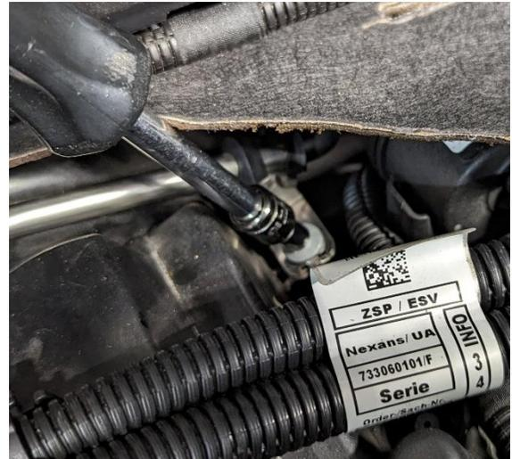
**Disclaimer:** The fuel pump is now accessible for removal, but take **CAUTION** as it is potentially under **EXTREME PRESSURE!** Safety glasses, a disconnected battery, and plenty of rags are highly recommended.
