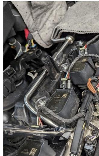
Once the engine fires up, check for leaks at each fuel connection point and double-check that the pump is torqued down. You can now re-clip the rear firewall covers, the harness bracket, the engine cover, and the DME cover. It's now time to make some power!
