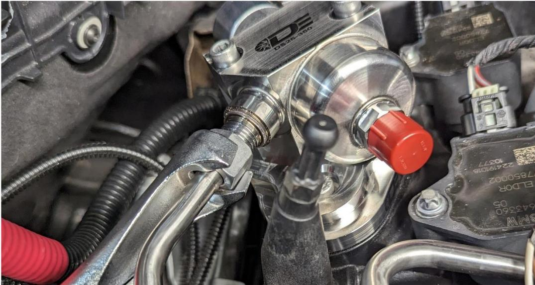
16. Install the Dorch electrical harness adapter as pictured below. Once clicked into place, be sure to push down the gray locking tab on the engine harness (the reverse of step 4).
