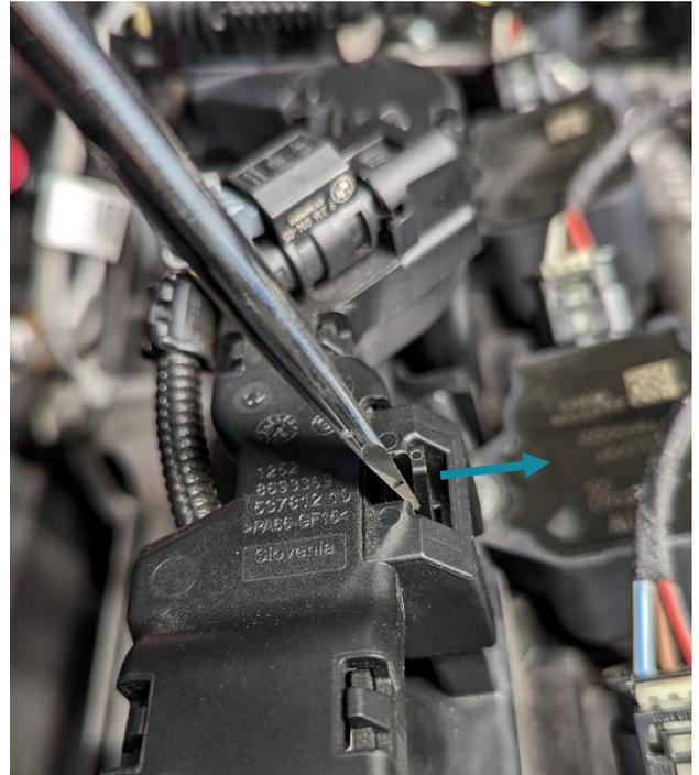
3. With the tabs released, the harness assembly will lift straight up and can be laid to the side out of the way:
