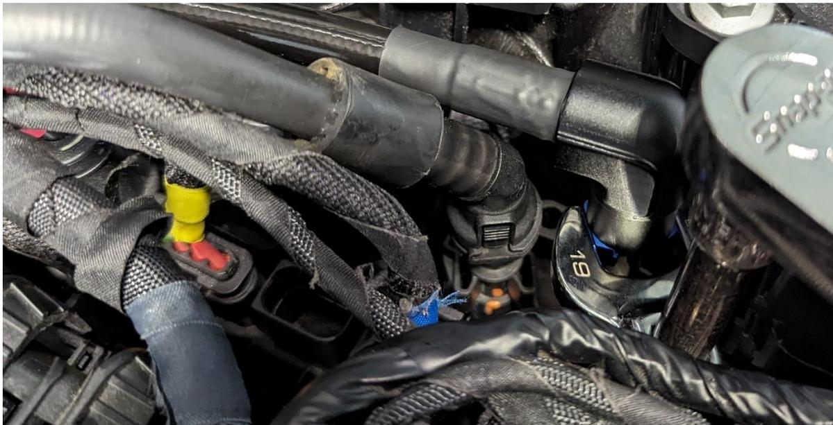
18. Route the hose behind the intake manifold just like the OEM hose and install it onto the HPFP **finger tight**. Using a 13mm socket, remove the rear cover hold down barb and reinstall it with the Dorch low pressure hose hold-down bracket:
