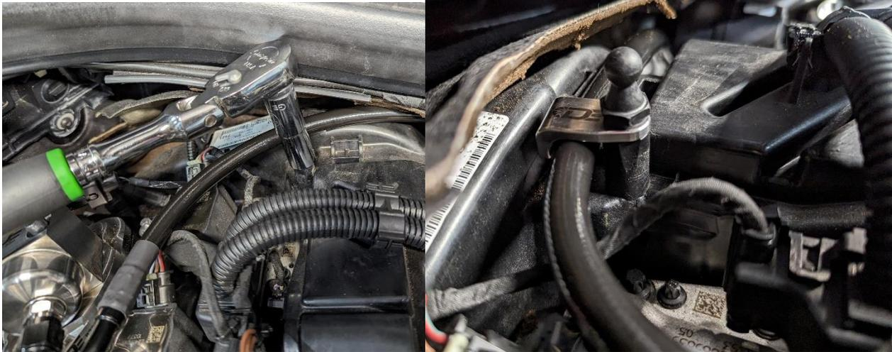
19. With the hose nicely tucked into the OEM groove location, you can now tighten the AN inlet fitting on the HPFP.
