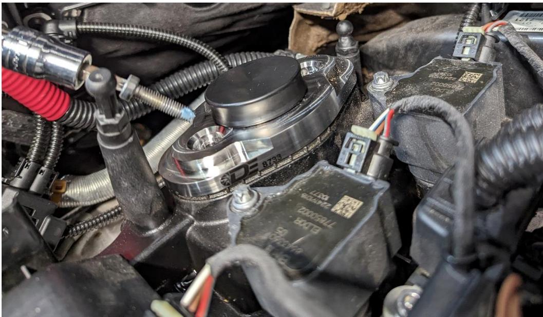
13. Remove the alignment tool and insert the Dorch Engineering fuel pump. Use extreme **CAUTION** when installing the pump. The pump's 5mm Allen bolts **MUST BE TIGHTENED EVENLY**. Uneven loading of the spring can damage the pump. Also, be **EXTREMELY CLEAN** as all HPFPs are very sensitive to contaminants.
