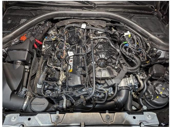
2. Next, remove the wiring harness bracket to gain access to the high pressure fuel line. This bracket has two tabs (circled below) that must be released by pushing outward:
