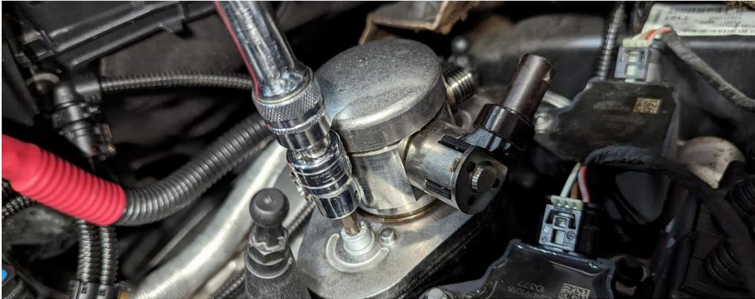
12. Install the Dorch Engineering pump flange using the supplied Torx T30 bolts and the flange alignment tool. Press the alignment tool into the center of the flange and tighten the bolts.
