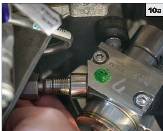
Fuel pump side high pressure spherical fitting and female line
